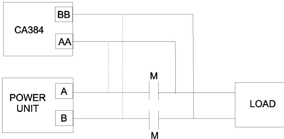
Dotted line connections may be used when the shunt field is fixed. Fixed shunt fields may be supplied either from constant potential rectifiers or shunt field regulators used as constant current regulators. (Shunt Field Temperature Compensation).
