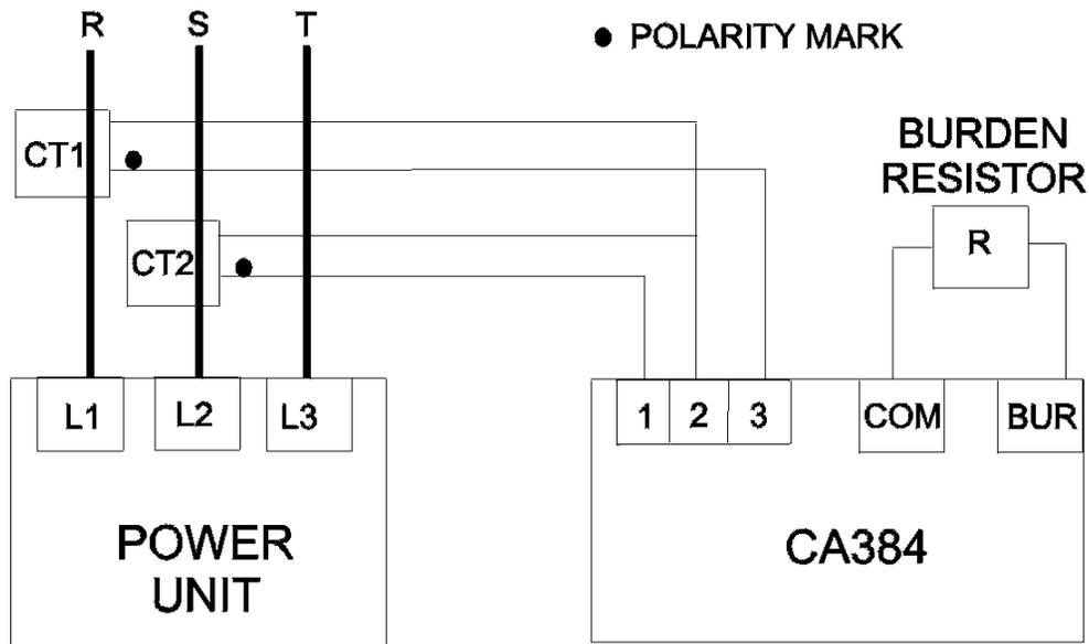
An external burden resistor (RBUR) is mounted on a 2-pole terminal strip at the top left on the CA384. The position is marked "BURDEN RESISTOR". Viewed from the component side of the CA384, the left terminal is zero common and the right terminal is the burden signal. A fixed internal burden is installed on the CA384. If no external resistor is installed, the current will be limited to a value less the 3% of the stack rating for +10.0VDC current reference into Terminal 11.
